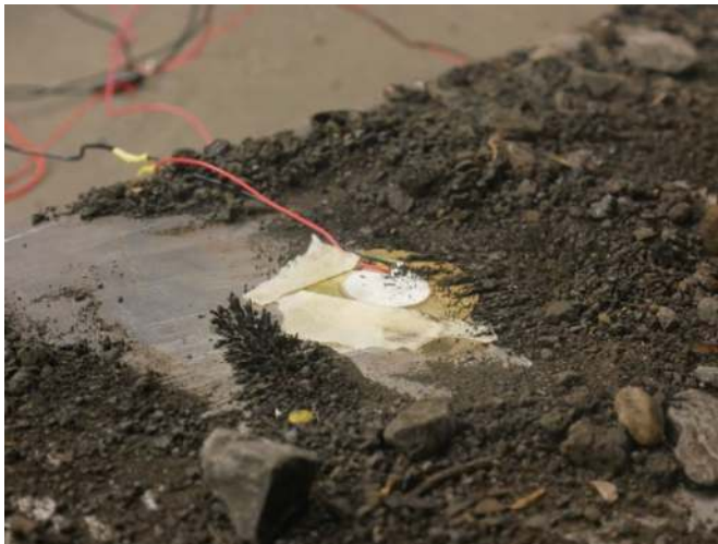
Figure 4. Close up of the piezo microphone in contact with magnetic soils in motion © Brice Ammar-Khodja
