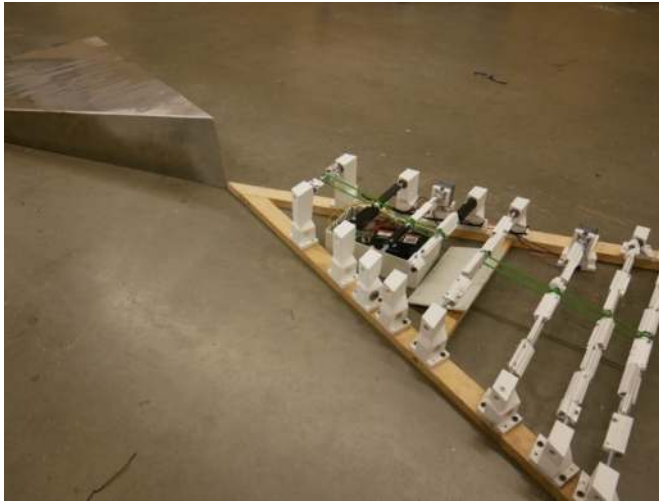
Figure 3. Kinetic system hidden in the sculpture's shell. The horizontal rods containing the magnets are activated by motors and driving belts. © Brice Ammar-Khodja
