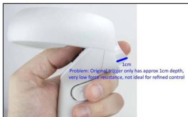
Figure 5. Inadequate trigger button of VR controllers, Shum, 2022.
